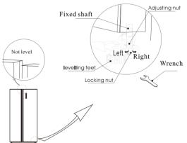
Before adjusting the height of the door, use a wrench to rotate the downward adjusting nut (shown above) counter clockwise for 2 turns. Rotate the upward adjusting nut allowing you to adjust the door height, followed by readjusting the downward adjusting nut to lock the door in its new position.
